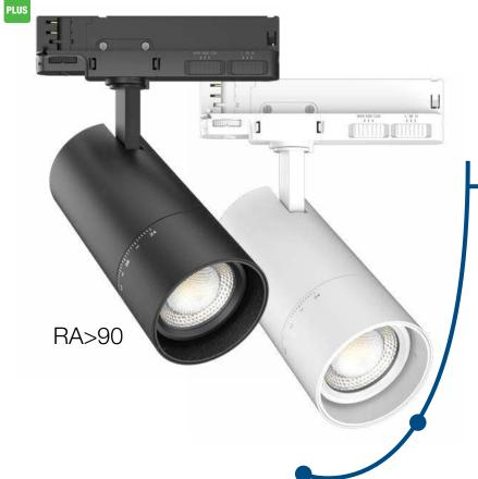
Two multi-power versions with the option of changing colour temperature, both operated by the selector switch located on the track adapter. Mechanical zoom for beam variation from 24° to 60°. Three-phase track adapter with integrated driver Robust die-cast aluminium construction Excellent colour rendering 3-year guarantee
